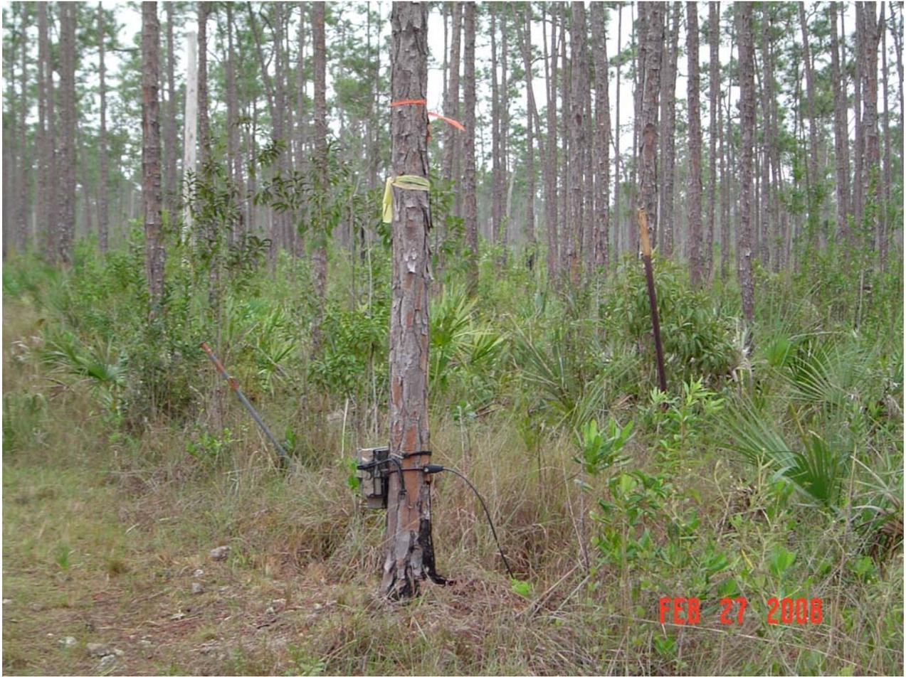
**Figure 2-2.** Image of camera unit on pine tree at survey station.
